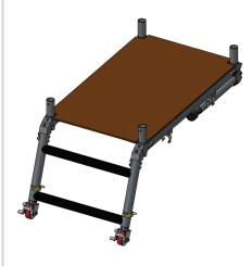
3. Unfold ladder legs one side at a time
