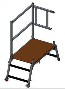
6. Rotate frame clip and use to secure side to platform.
